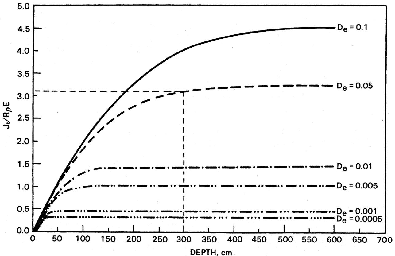
FIGURE 4. Normalized Surface Flux Versus Tailings Depth
