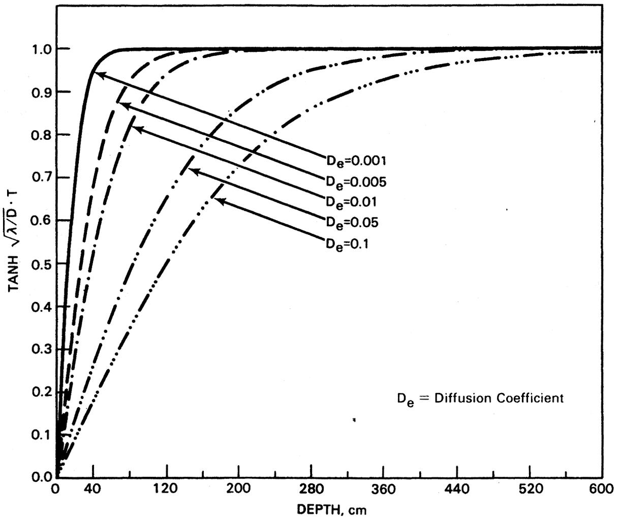
**FIGURE 3.** Effect of Ore Pile Thickness on Hyperbolic Tangent Term in Radon Flux Equation
