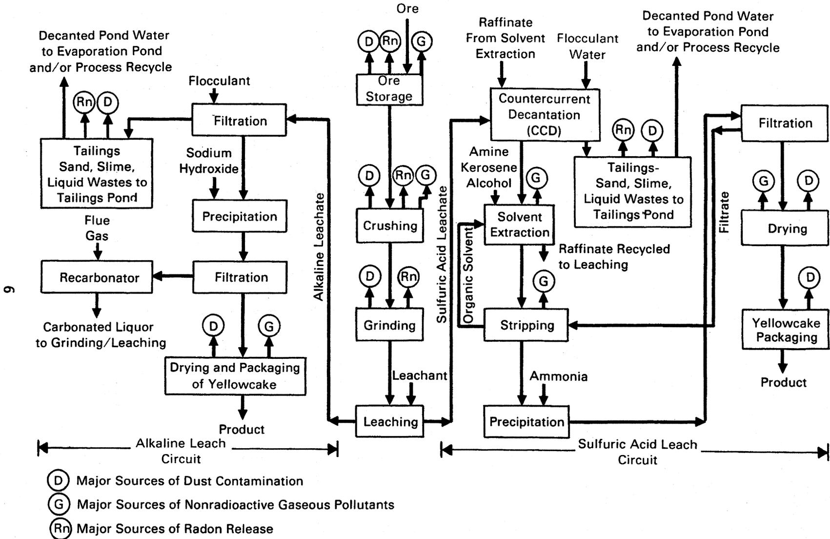
FIGURE 2. Major Source Pathways for Uranium Milling Processes
